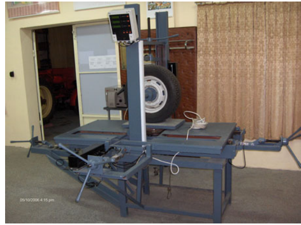
Laboratory installation for tire testing
